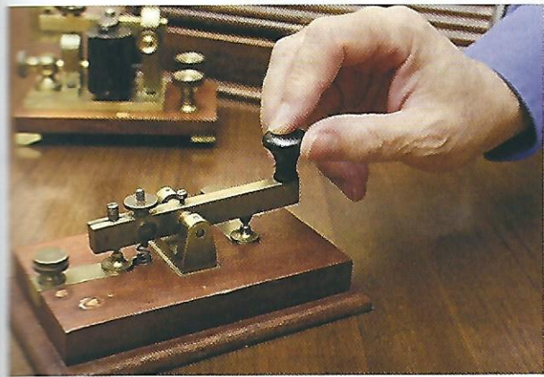
The telegraph key is a switch that opens and closes a long-distance electric circuit, transmitting signals—the dots and dashes of a coded alphabet—by wire.
